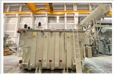
132 KV, 20/25 MVA Power Transformer for Agra Metro
